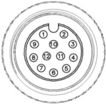
12 pin assignment on camera
