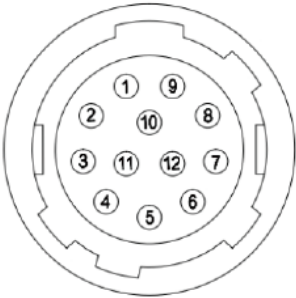
Port definitions of 12-pin signals
